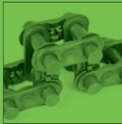
Install outer flat link
