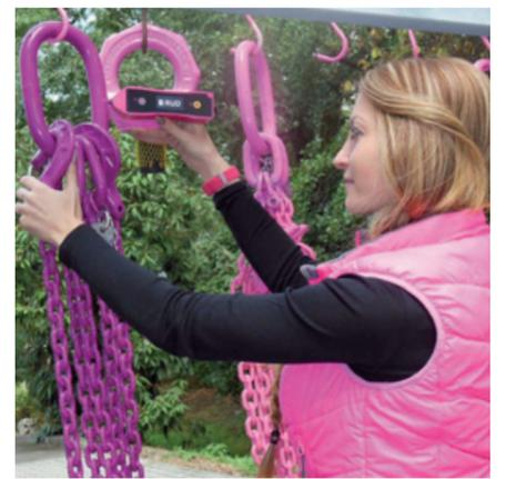
*Even in the harshest of environmental conditions, such as those found in deep and open-cast mining, or in contact with pit water or saltwater, or in sand-blasting processes, the identification data could still be read from the chips in the field without any problems.*
