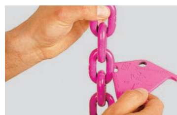
Testing wear of nominal dia.
