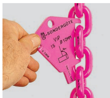
Testing for plastic elongation caused by overload
