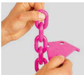
Testing wear of nominal diameter
