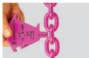
Testing for elongation caused by wear of nominal diameter.
