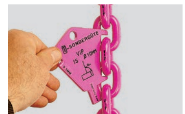
Testing for pitch elongation caused by overload.
