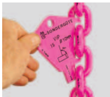
Testing for plastic elongation caused by overload
