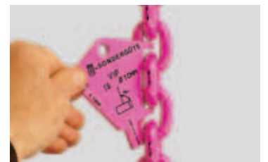
Testing for pitch elongation caused by overload.
