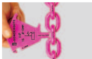
Testing for elongation caused by wear of nominal diameter.
