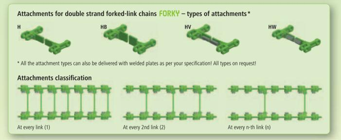
Forked-link chains are suitable for transporting powdered, flaky, grainy and fragmentary bulk materials, but not for sticky or baking bulk materials.
