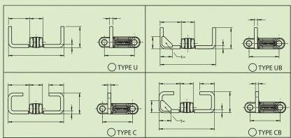
Type U and UB (UB is custom-made) for high ascending transport, 10° up to 25° Type C and CB (CM is custom-made) for high ascending transport and dusty material, 10° up to 25°
