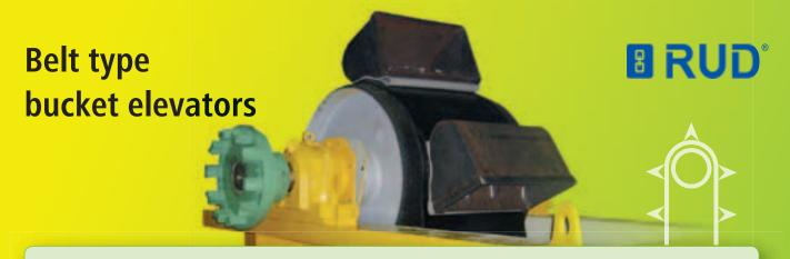
Belt type bucket elevator designs using textile or steel reinforced belts transport materials dust-free without difficulty, even to great heights and are especially suitable for the continuous vertical conveyance of free flowing bulk materials. Suitable adaptations are made to handle coarse-grained or higher temperature materials.
