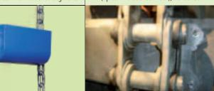
Central chain bucket elevators for large conveyance capacities, coarse dry bulk materials (clinker, gravel, circulating goods and cement granules) and high speed (up to 1.7 m/s); steel chain bucket elevators.
