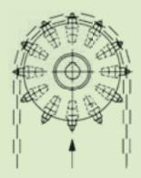
In case of replacements: here, replace individual teeth without taking off the chain.
