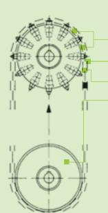
The welded joints of the (vertical) chain links must point at the wheel centre.
