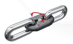
Turn the locking pin through 90° by means of a hex wrench. When turning you must feel a hard point in order to positively locking the pin
