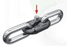
Insert the locking pin flush into the connector. Be aware of the position of the cam - in parallel to the flights of the inner sides of the connector schackles.
